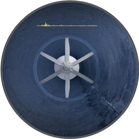
PipeDiver navigates in-line valves, sharp bends, and tees
