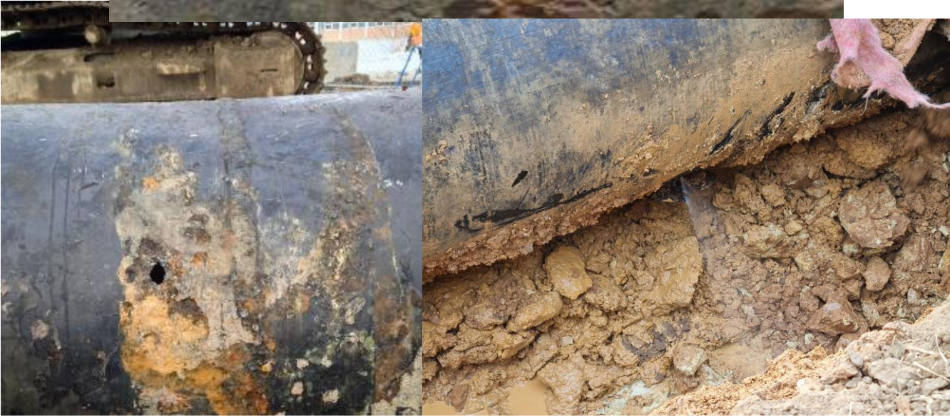
Mettalic Pipes – Pitting, cracking & Leaks
